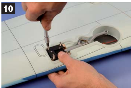
10 Visser le train en place (nous recommandons des vis auto-tarandantes 2,9x16mm 1310516). Attach the retract in place (we recommend to use self tapping screws 2,9x16mm #1310516).
